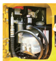
Fuel Feed Pump
